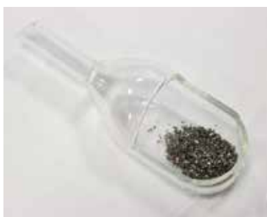
Fig. 6 above: Fine powder needs to be placed in a capsule before analysis in the ONH-p2.
