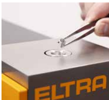
Fig. 7: Application of a nickel basket (flux for precious metals and refractories). Here without the nickel capsule and sample.
