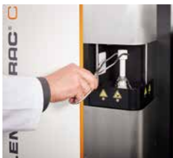
Fig. 5: Placing sample with accelerator on the pedestal of the ELEMENTRAC CS-i
