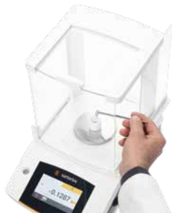
Fig. 4: Applying accelerator to a weighed sample
