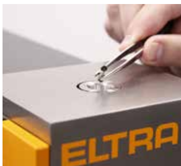
Fig. 9: Application of open capsule with powder
