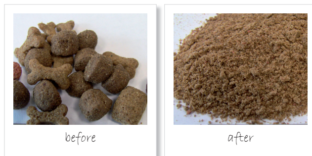
Figure 4: Homogenization of dog food pellets before and after grinding down to < 0.5 mm in the ZM 200
