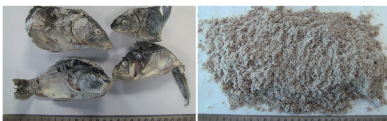
Figure 9. Homogenization of fish; from left to right: original sample, sample ground to <1 mm.
