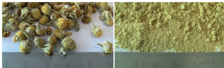
Figure 10. Homogenization of chamomile; left to right: original sample, sample ground to <100 \mu\text{m} .
