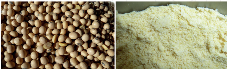
Figure 14. Homogenization of soy beans; left to right: original sample, sample ground to <500 \mu\text{m} .
