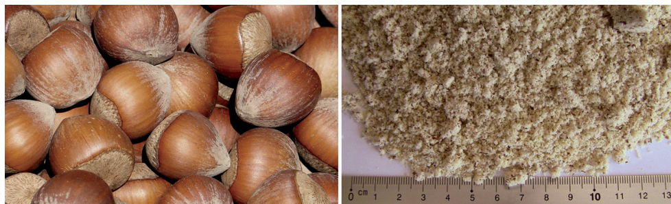
Figure 7. Homogenization of nuts; from left to right: original sample; pulverized sample of <300\ \mu\text{m} .
