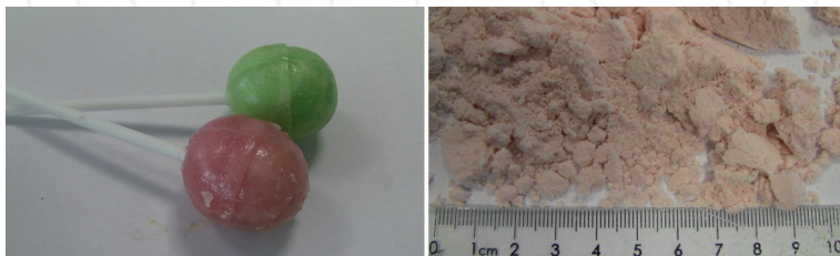
Figure 13. Homogenization of candy; left to right: original sample, sample ground to <500 \mu\text{m} .
