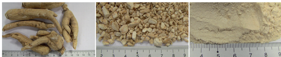
Figure 11. Homogenization of ginseng; left to right: original sample, sample ground to <8 \text{ mm} , sample ground to <100 \mu\text{m} .
