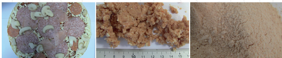
Figure 1. From left to right: a whole pizza; sample after grinding to coarse particles of <5 mm; fully homogenized sample with particle sizes of <0.5 mm.
