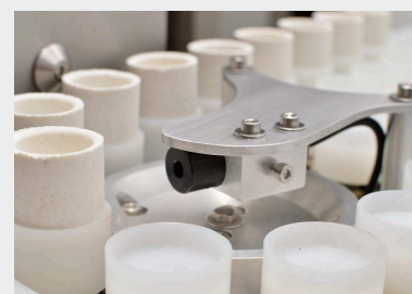
Autoloader with acid-resistant plastic crucible holders
