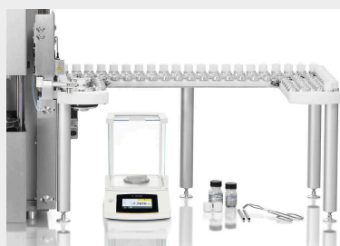
Autoloader with 130 crucible positions
