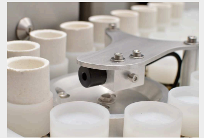
Autoloader with acid-resistant plastic crucible holders
