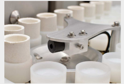
Autoloader with acid-resistant plastic crucible holders
