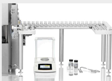
Autoloader with 130 crucible positions
