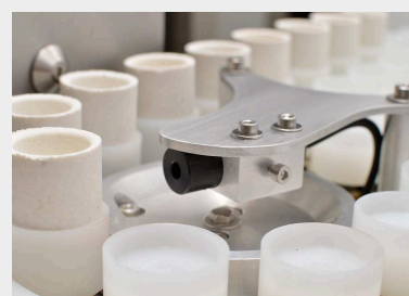
Autoloader with acid-resistant plastic crucible holders
