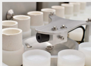
Autoloader with acid-resistant plastic crucible holders
