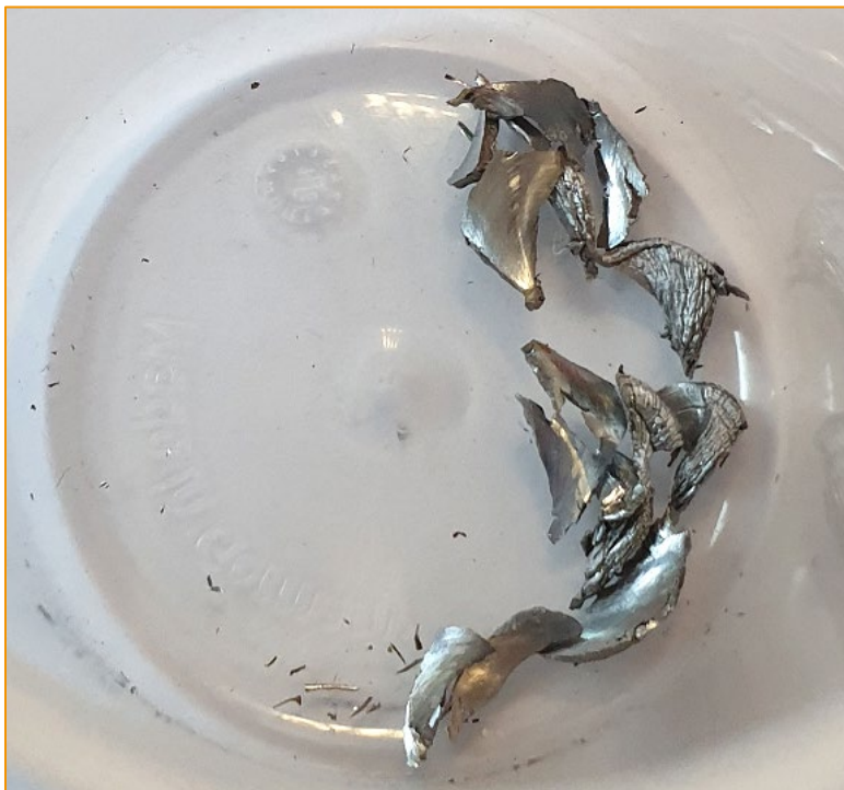
Illustration of a critical sample shape: Maybe not applicable in furnace and crucible
