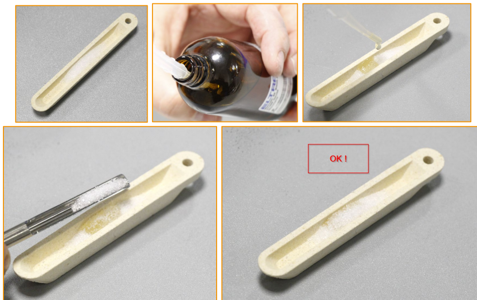
Analysis procedure for analyzing liquid samples like oil
