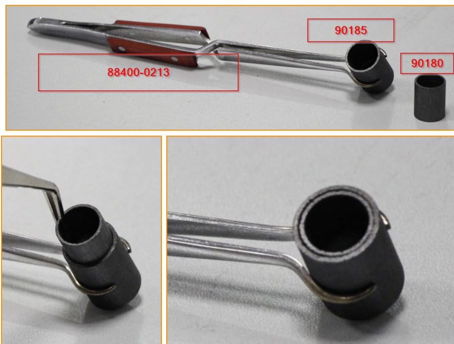
Illustration of usage of inner and outer crucible
