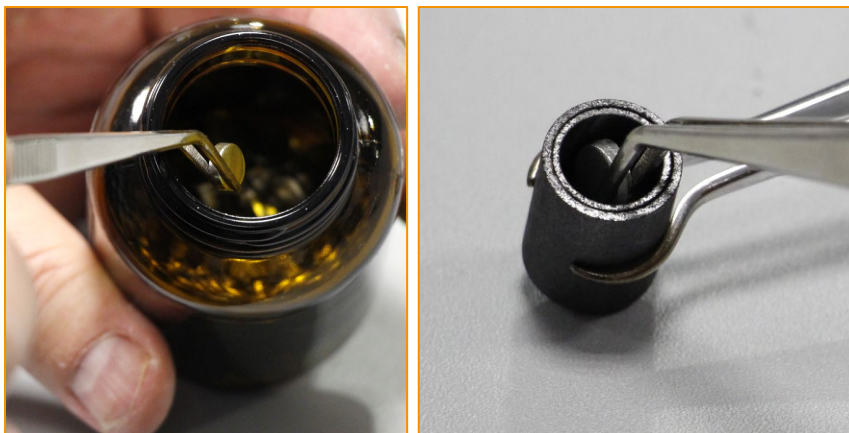
Application of tin pellets to a graphite crucible (H in titanium analysis)
