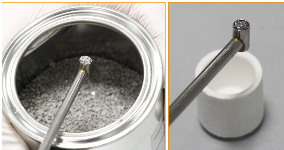
Application of tungsten with spoon (part number 23113)
