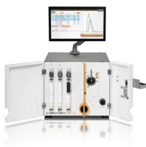
Fig. 4: ELEMENRAC CHS-r with optional monitor holder and touchscreen
