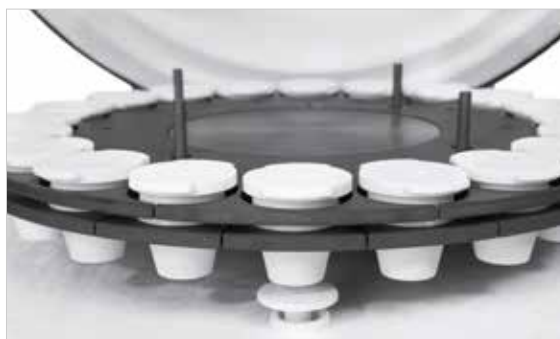
PC-controlled application of crucible lids / crucibles closed
